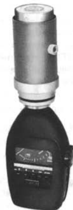
Figure 5-2. Type 1562 Calibrator mounted over SLM Microphone.
